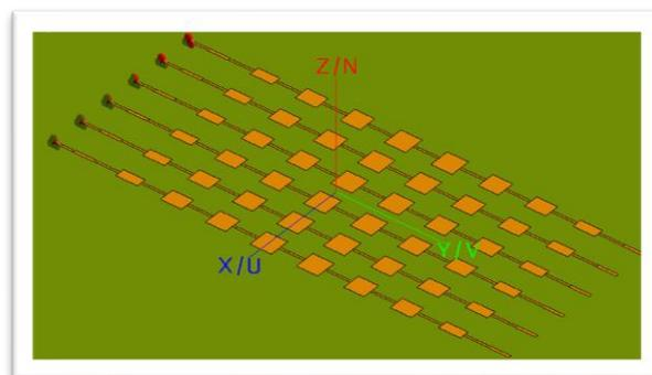
Fig. 1. Microstrip Patch antenna array with 6 columns.
