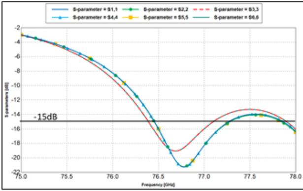
Fig. 2. Return loss of individual array columns in the radar.
